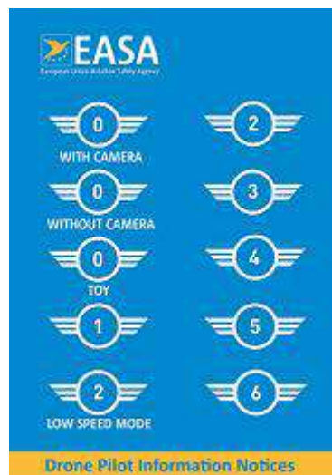
Figure 1 C-Marking Labels as per regulation 2019/945 (EASA, 2022)
