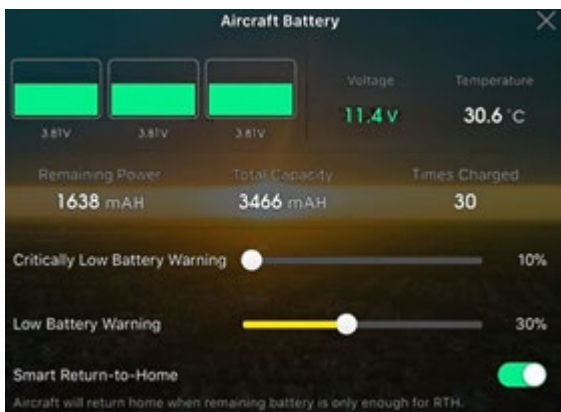
Figure 5 Battery cells levels (displayed in Volt units)
