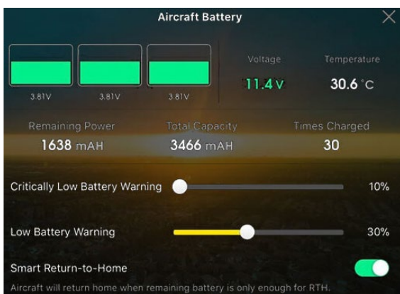
Figure 31 Battery cells levels and settings expressed in Volts.
