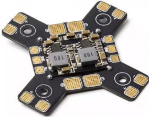
Figure 26 Drone power distribution board - hobbyking.com
