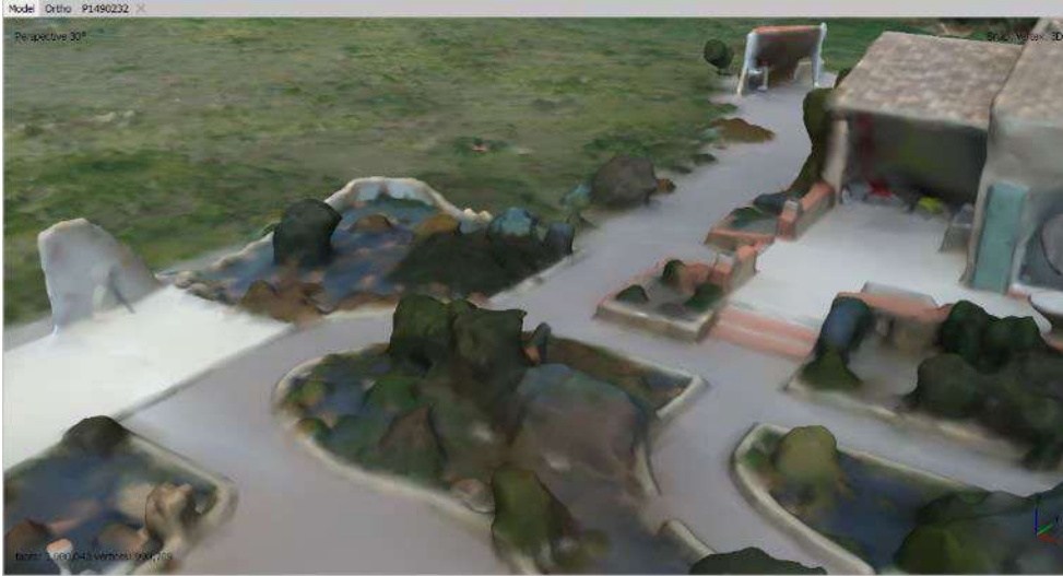
Figure 6-2 mesh made with "medium" face count
