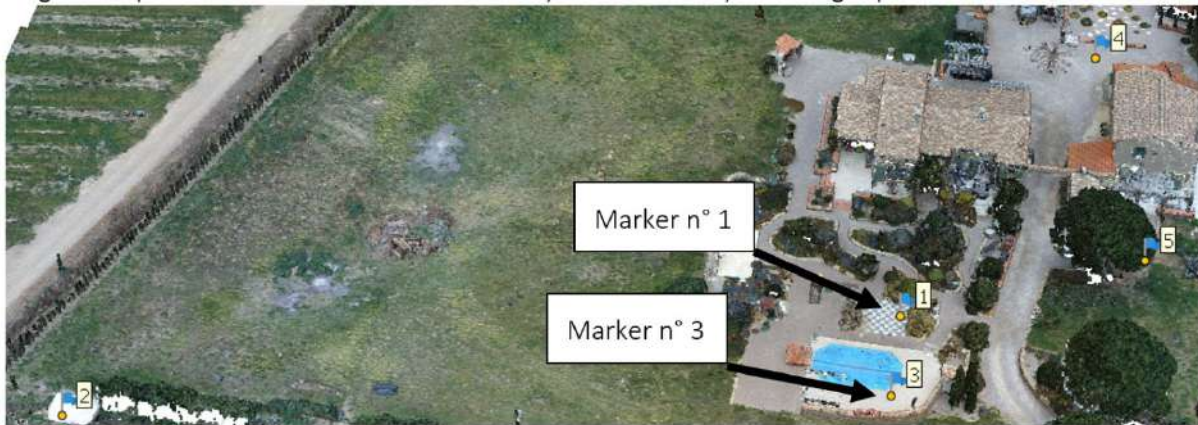
Figure 5-14 markers created on the point cloud
