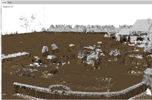
Figure 8-9 dense cloud ground class points seen close: walls are in the wrong class because of the "1m max distance" set
