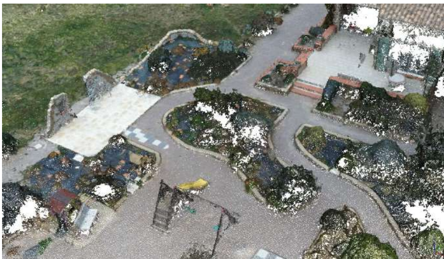
Figure 5-4 Metashape point cloud with white gaps where no point was built
