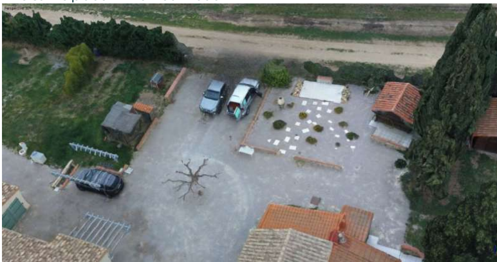
Figure 8-15 tiled model showing all the items removed by classification to obtain the DTM
