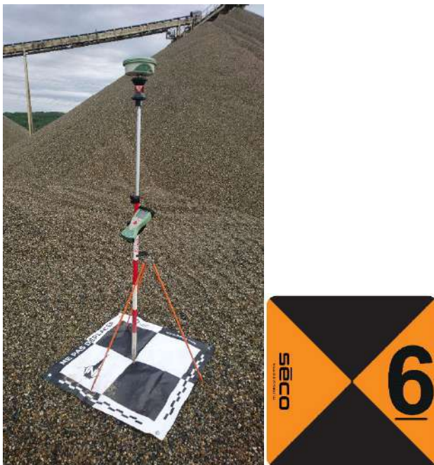
Figure 3-6 ground geolocation target surveyed by GNSS
