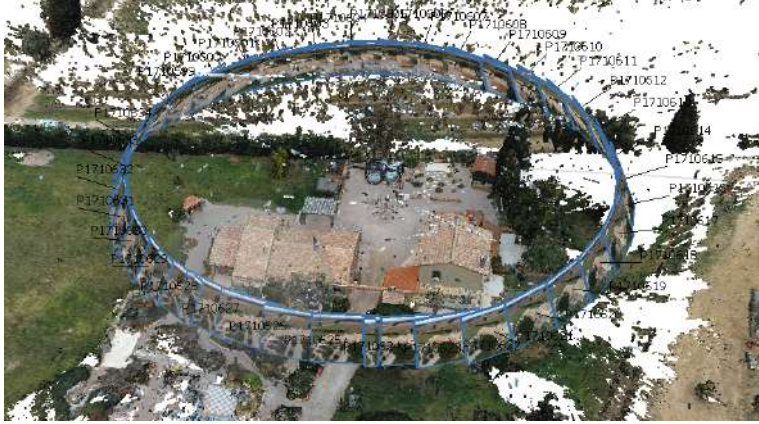
Figure 3-5 circular drone flight for 3D building photogrammetry
