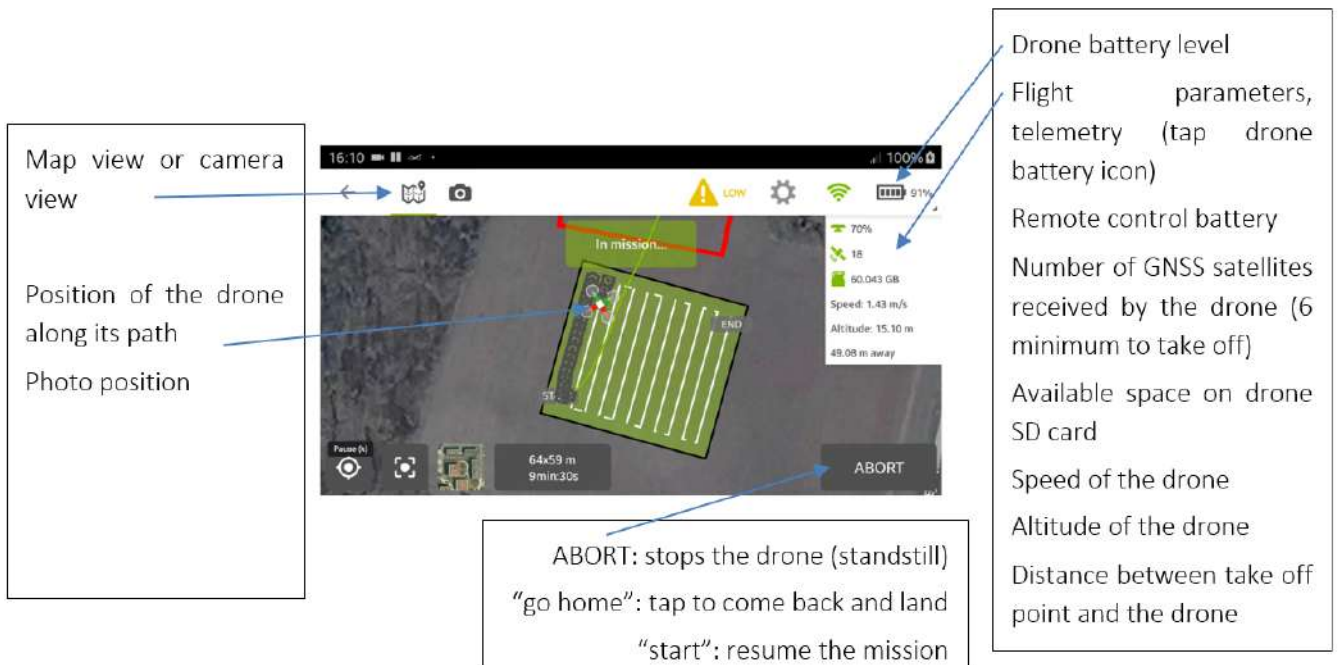
Figure 4-5 Pix4DCapture mission display while the drone is flying
