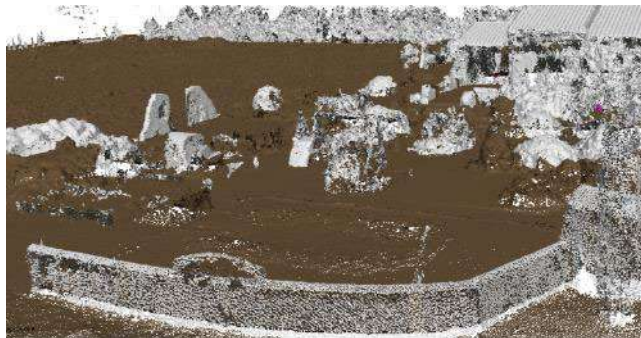
Figure 8-10 dense cloud ground class correct points
