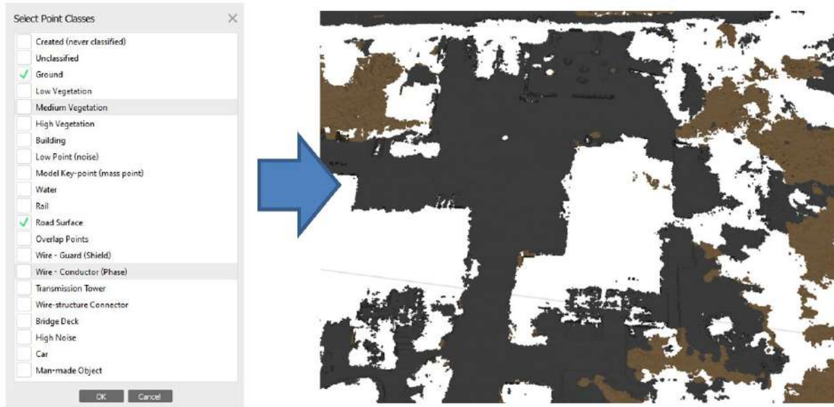
Figure 9-6 point cloud displaying only ground and road surface
