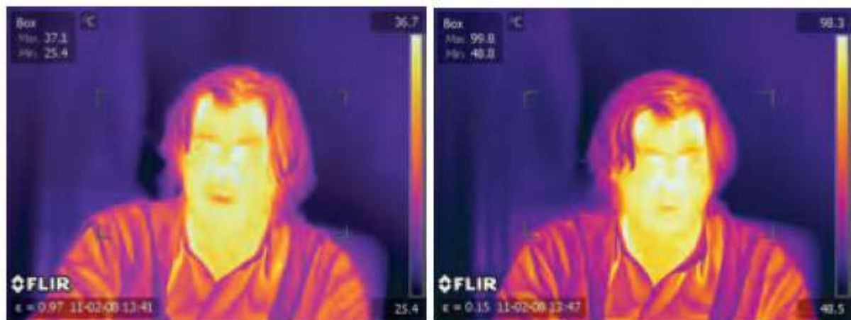
Figure 4-2: Emission Value (FLIR Systems)
