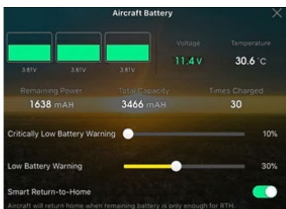
Figure 5 Battery cells levels (displayed in Volt units)
