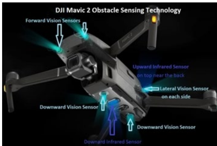
Figure 21 Proximity sensors on a drone (drone-festival.com)
