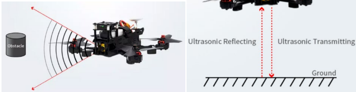
Figure 20 vertical and horizontal ultrasonic sensing - microcontrolertips.com
