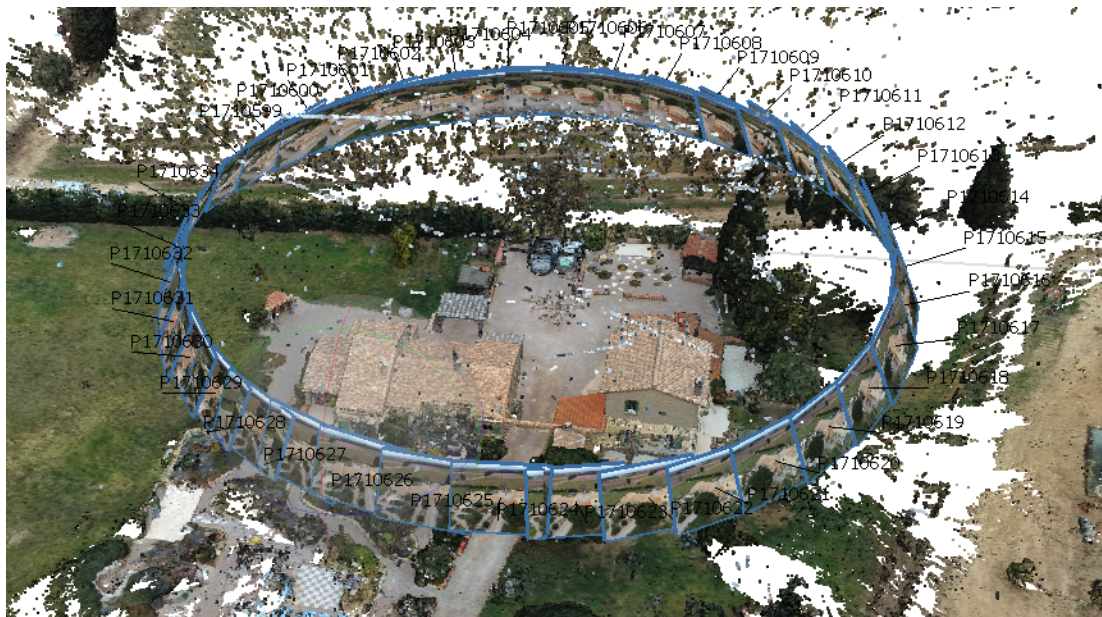
Figure 6-7 travelling around a building for 3D photogrammetry
