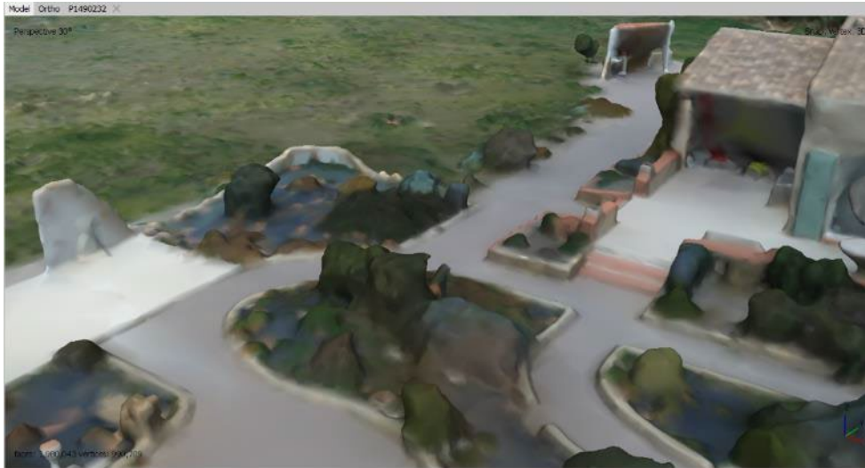
Figure 6-2 mesh made with "medium" face count
