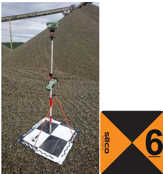
Figure 3-6 ground geolocation target surveyed by GNSS
