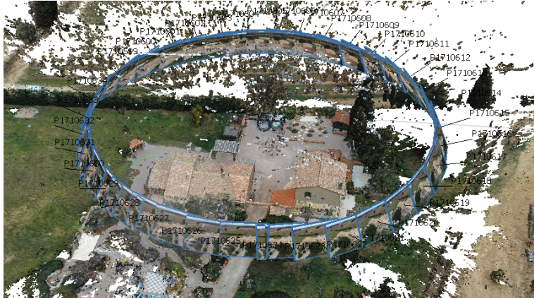
Figure 3-5 circular drone flight for 3D building photogrammetry
