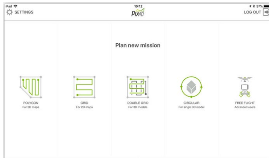
Figure 4-3 Pix4DCapture flight path selection
