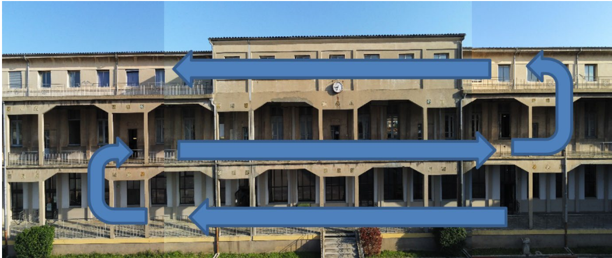
Figure 3-10 path for façade photogrammetry
