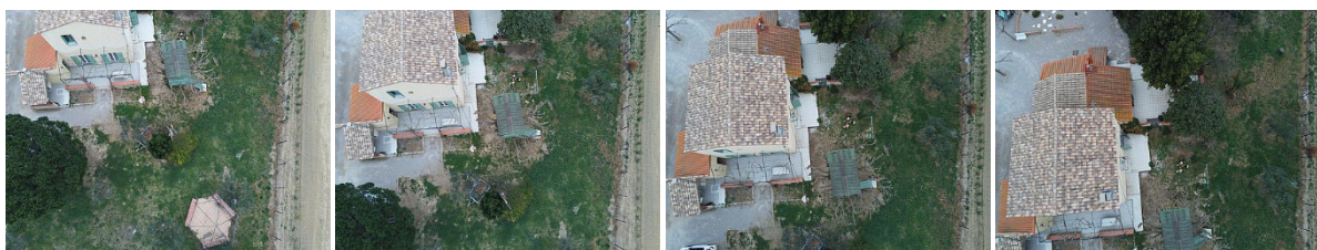
Figure 3-4 photo sequence with good overlap and camera tilt
