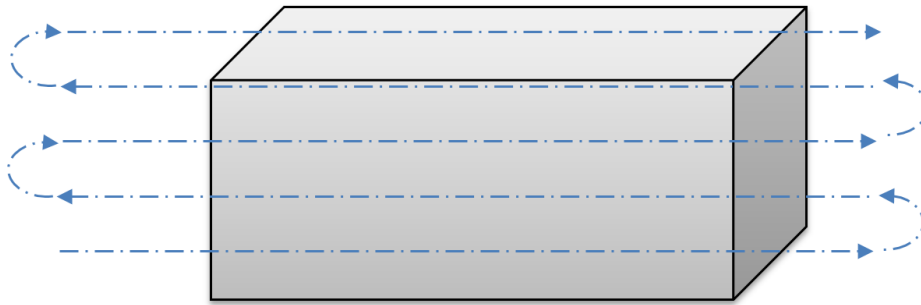
Figure 3-15 path for façade and 3D building capture
