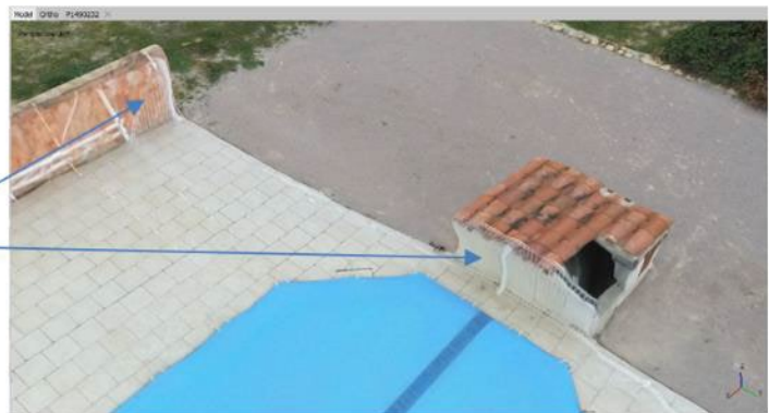
Figure 6-12 tiled model defaults on the pool's wire fence
