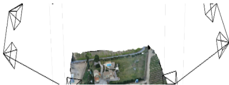
Figure 10-7 camera movement with 10 key frames and no smooth camera track
