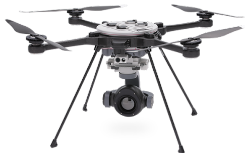
Figure 2-22 FLIR SkyRanger R70 (www.flir.eu)
