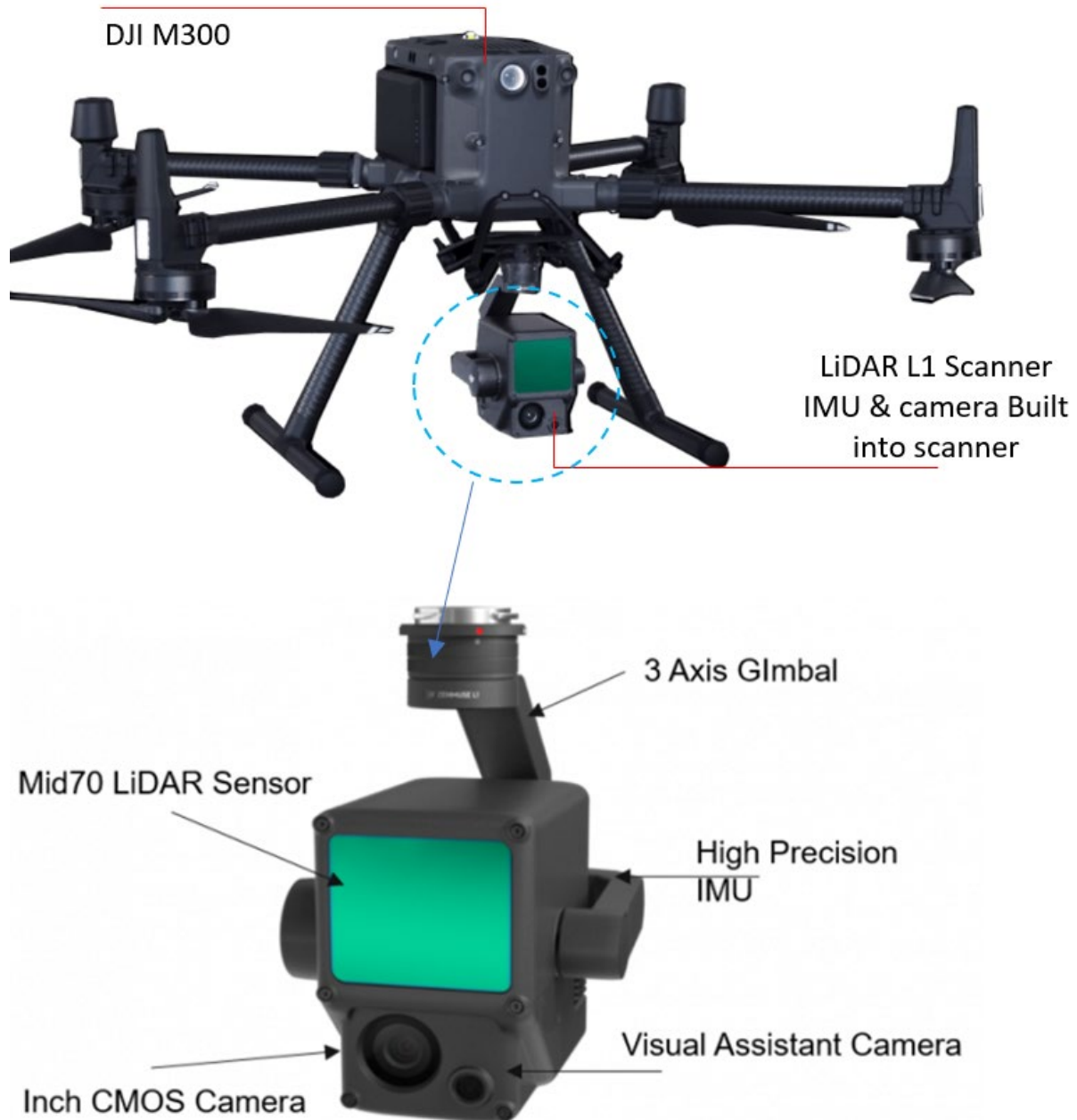
Figure 7 Multi Rotor DJI M300 with L1 Laser Scanner 17
